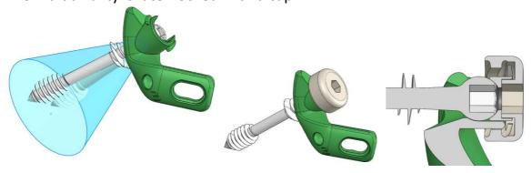
The facet screws, thanks to the presence of two threads with slightly different pitches, gently compress both opposite massif of the facet, optimizing stability and bone fusion.
